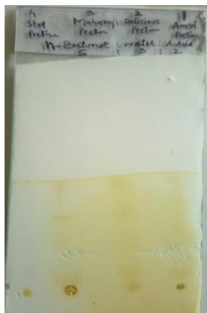
Figure 1. TLC profile of extracted pectin with reference to that of standard pectin
