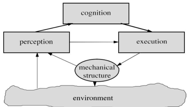
Figure 2: Major functions of an intelligent machine system
